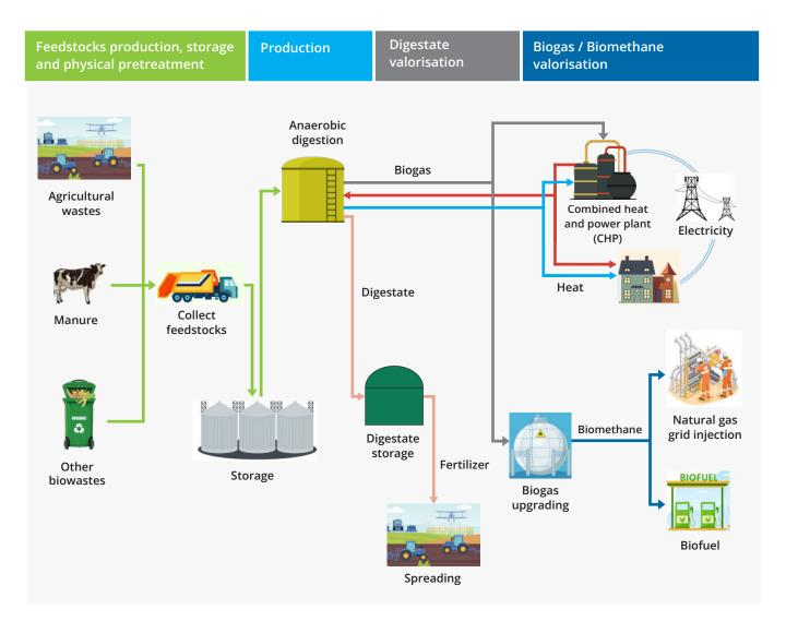
Anaerobic digestion is a process through which bacteria break down organic matter in the absence of oxygen.
